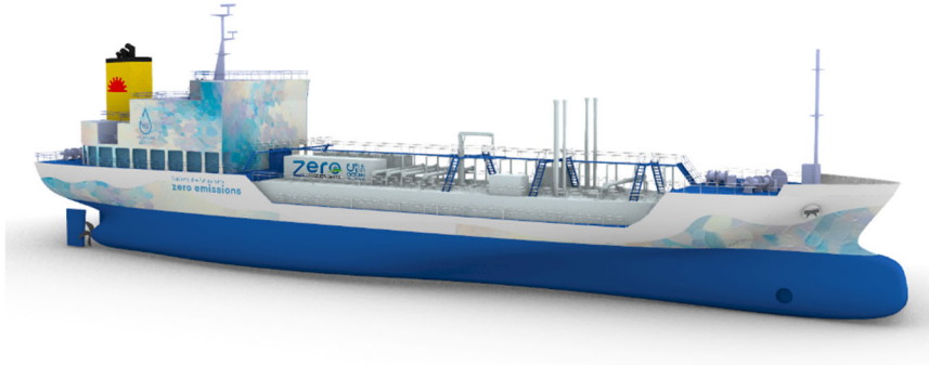
Rendering of hydrogen fuel engine electric propulsion ship. (Ship color to be decided.)
