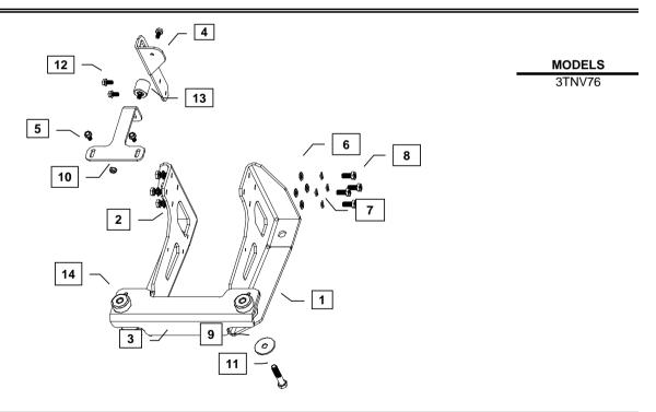
Remarks: (A) 26106-100202 is a service part used to replace the bolt, lock washer and washer assembly (items: 6, 7 and 8).
