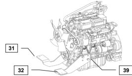
2. Fasten each engine foot (38) to the front engine mounting pad with the M10 X 1.5 - 25mm bolts provided (40). KF6 engine foot shown.
