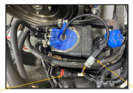
Coolant Control Valve (117A) DEF Tank Plug (117B)
