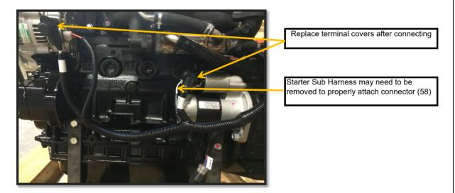
Layout harness as shown. Connectors 1, 2, 64, 65 - 66, 44, 48, 101 - 104, and the battery leads (49 & 50)
