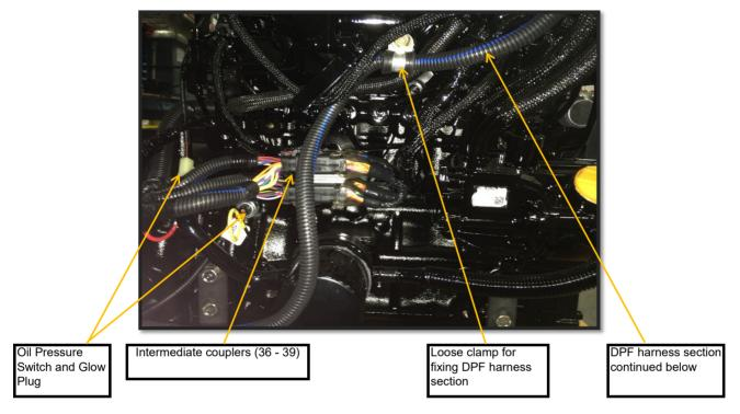
6. Route the DPF branch between the EGR valve and the fuel filter up to the DPF connections. Check and adjust if necessary to ensure that no contact will be made in operation between harness and high temp surfaces (DPF, etc)
