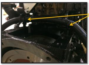
P-clips hold down the alternator and starter section of loom to the flywheel housing. Make sure P-clips and loom have the proper orientation to allow the loom to rest close to the flywheel barrel.
