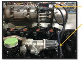
The routing shown if for exhaust manifold mounted DPF's. Flywheel mounted DPF's will need harness section routed similarly. This section is secured by clamp shown above.
