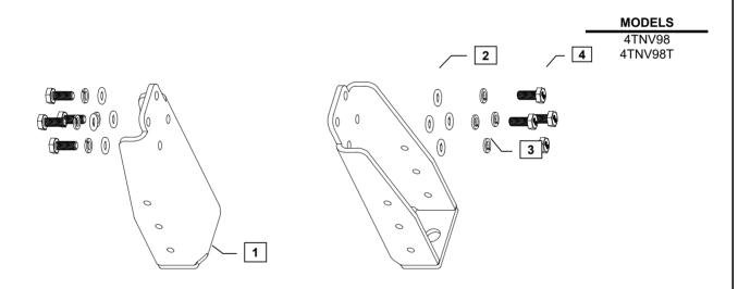
Remarks: 1 (A) 26106-100202 is a service part used to replace the bolt, lock washer and washer assembly (items: 2, 3 and 4).
