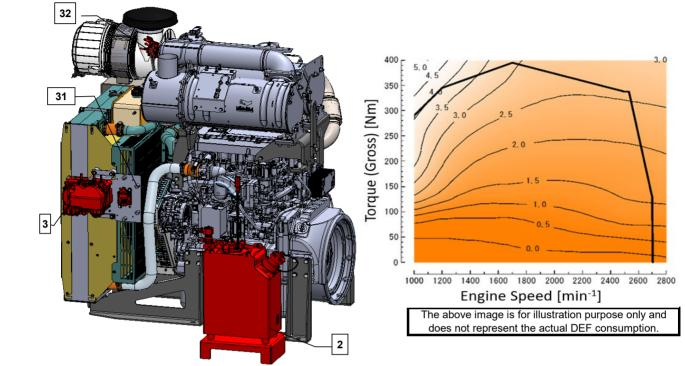
WARNING: As EPA requirement, for regulation applied area, set the urea water tank capacity so that the urea water replenishment timing to the urea water tank is adjusted such that the refueling of fuel is performed at least once for one urea water supplementation, even in the operating condition with the worst urea water consumption amount.
