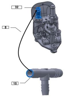
12 Cut the Hose, 1/2" ID (10) provided in the DEF kit to precise length **1677 mm**, and attach it to the Tee Fitting (15) and the Coolant Control Valve (3) using Hose Clamps (12). Ensure the coolant line is well connected to prevent leaks.
