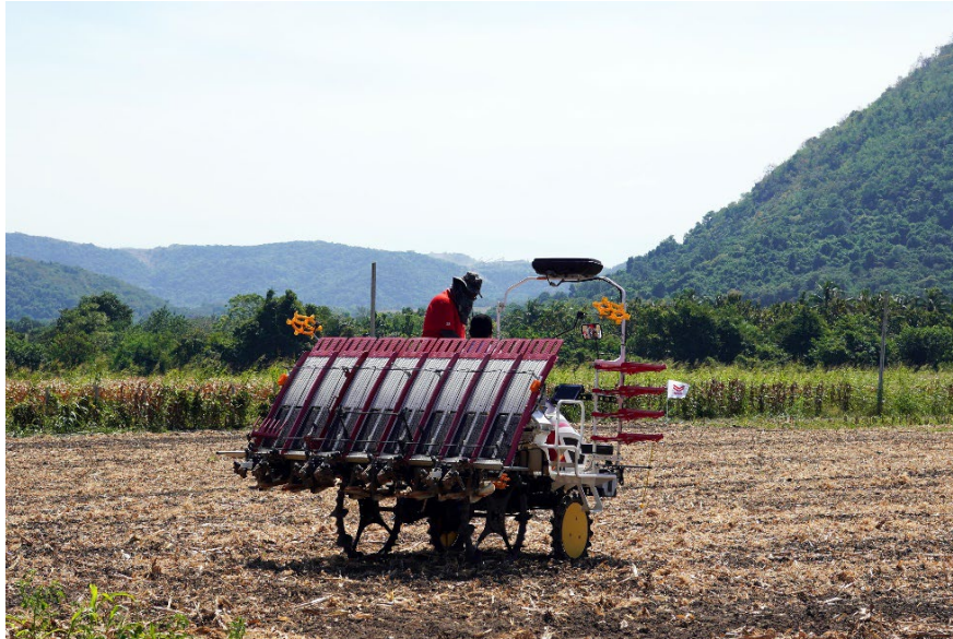
Rice transplanter with automatic turn steering.
