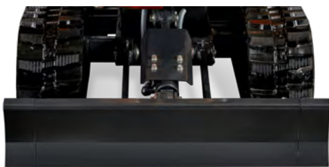
Extended undercarriage 840 mm - Increased stability
