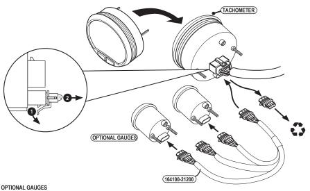
Fuel Gauge - 164100-53220 Oil Pressure Gauge - 164100-53210 Water Tempurature Gauge - 164100-53200
