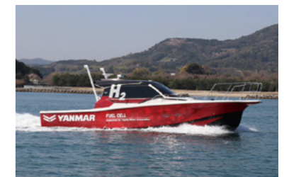
Test boat with maritime fuel cell system
