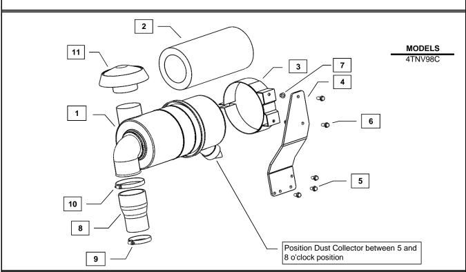
Note: Part codes are not assigned to non-servicable component parts.
